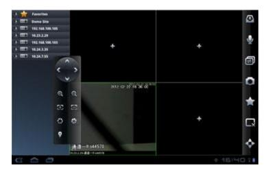
• When the playback window is in full-screen mode, you can use your hand gesture to realize PTZ or EPTZ operation.
